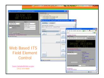
Using a web browser and carefully selected commercially available hardware components, design a system to control a remotely located ITS field element.
